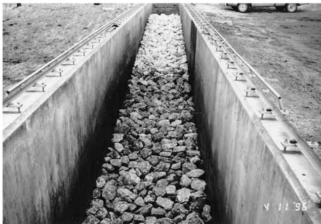
Figure 3—The 1.83 m (6.00 ft) wide flume with D<sub>50</sub> = 188 mm (0.617 ft) and S = 8%.
