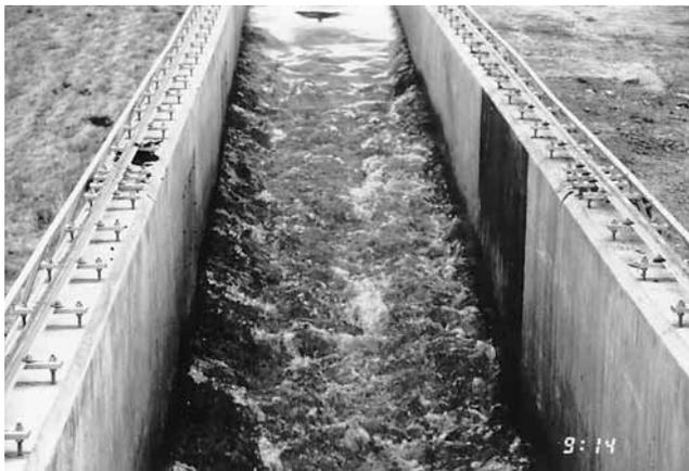
Figure 5—Flow in the 1.83 m (6.00 ft) wide flume:  $q = 0.69 \text{ m}^3/\text{s}/\text{m}$  ( $7.43 \text{ ft}^3/\text{s}/\text{ft}$ );  $D_{50} = 188 \text{ mm}$  ( $0.617 \text{ ft}$ );  $S = 8.0\%$ .
