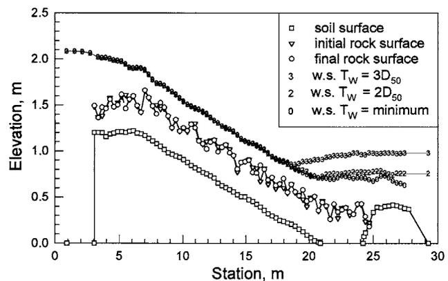
Figure 7—Bed and water surface profiles: 1.83 m (6.00 ft) wide flume;  $q = 0.752 \text{ m}^3/\text{s}/\text{m}$  ( $8.09 \text{ ft}^3/\text{s}/\text{ft}$ );  $D_{50} = 188 \text{ mm}$  ( $0.617 \text{ ft}$ );  $S = 8\%$ . (water surface at the tailwater).
