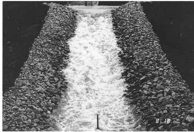
Figure 6—Flow in the field flume:  $q = 0.44 \text{ m}^3/\text{s}/\text{m}$  ( $4.74 \text{ ft}^3/\text{s}/\text{ft}$ );  $D_{50} = 188 \text{ mm}$  ( $0.617 \text{ ft}$ );  $S = 16.7\%$ .
