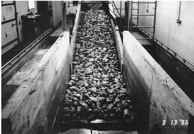
Figure 2—The 1.07 m (3.51 ft) wide flume with D<sub>50</sub> = 89 mm (0.292 ft) and S = 22.2%.
