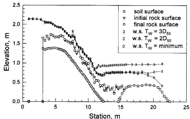
Figure 8—Bed and water surface profiles: 1.83 m (6.00 ft) wide flume;  $q = 0.35 \text{ m}^3/\text{s}/\text{m}$  ( $3.77 \text{ ft}^3/\text{s}/\text{ft}$ );  $D_{50} = 188 \text{ mm}$  ( $0.617 \text{ ft}$ );  $S = 22.2\%$ . (water surface at the tailwater).
