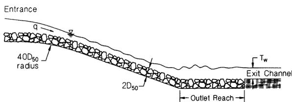
Figure 1—Typical rock chute profile.
